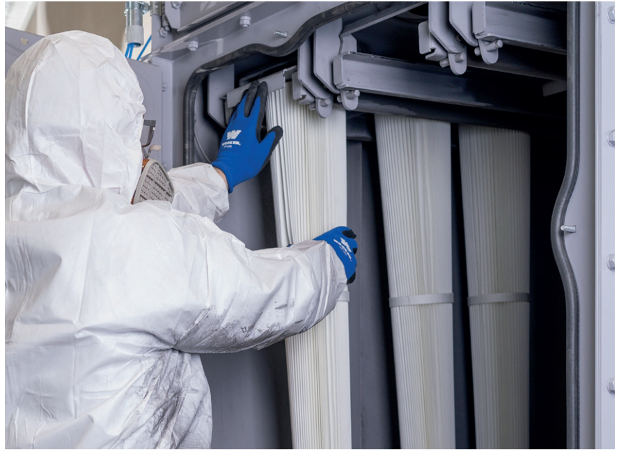
Filter system with quick-release fastener
