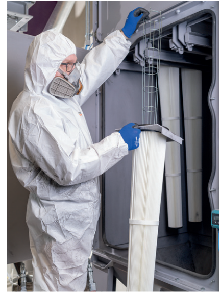
Conical filter cartridges with separate support basket
