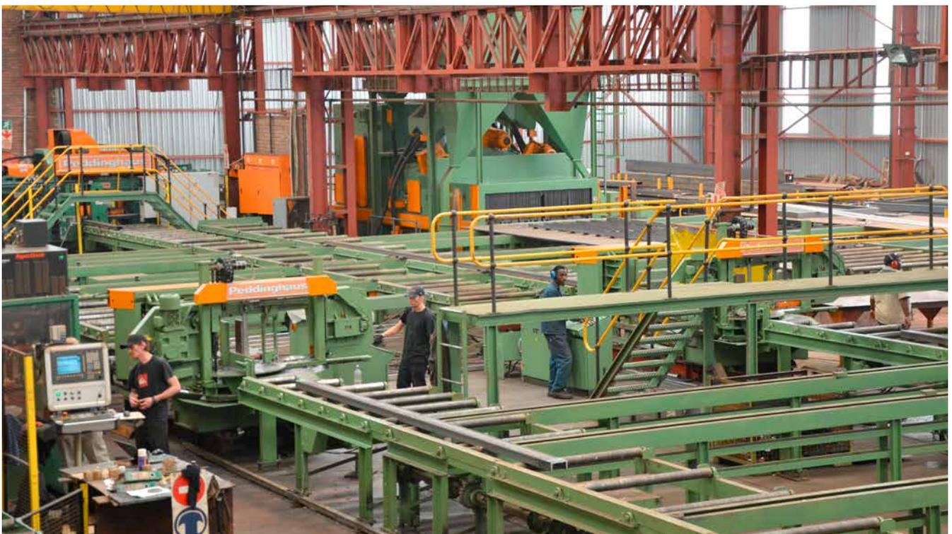
Blast machine with cross conveyor
