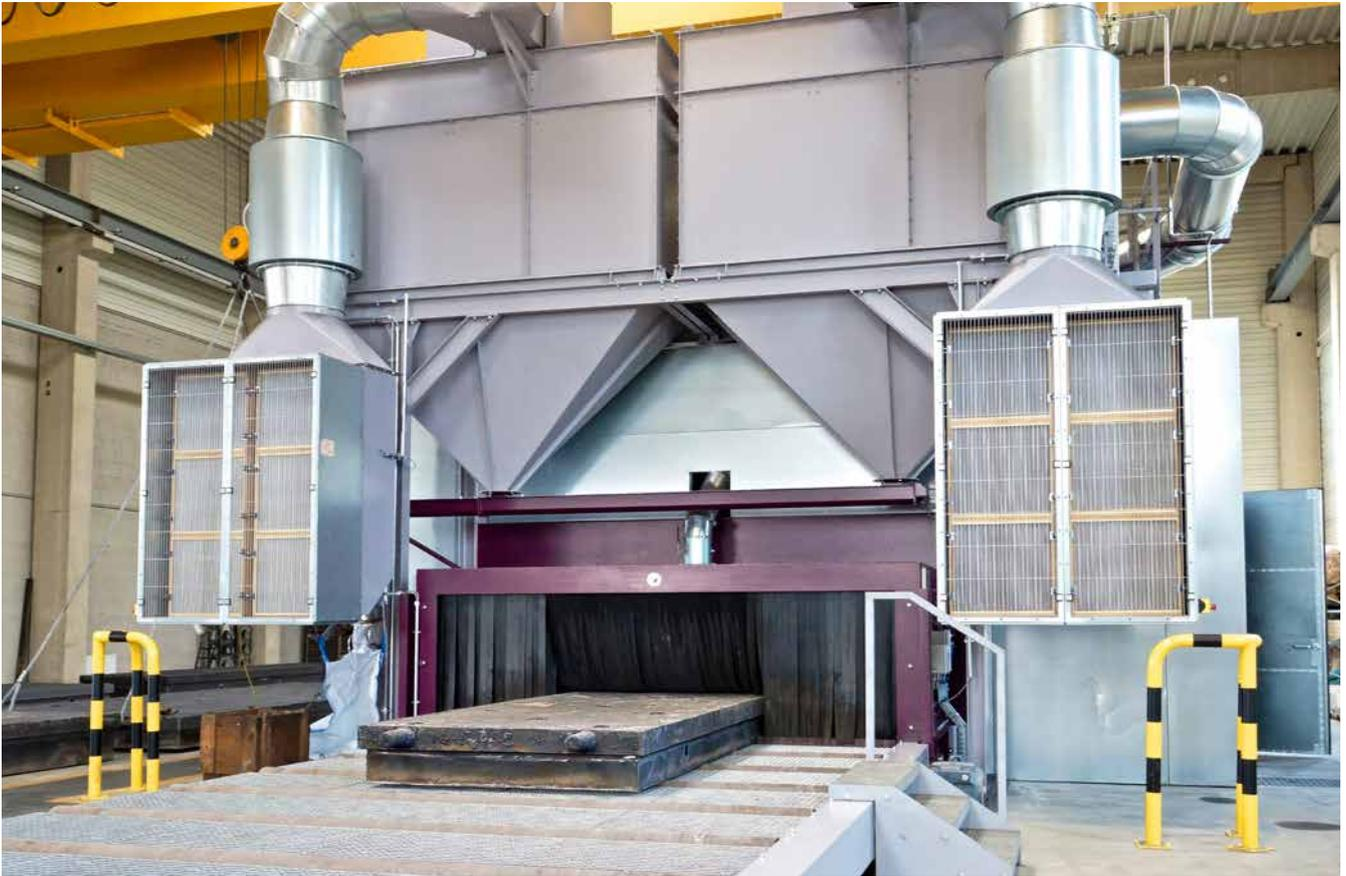
**AGTOS** manufactures roller conveyor shot blast machines also as special machines. The machine shown here is designed for the processing of cast clamping plates, measuring plates and testing plates weighing up to 25 tons.
