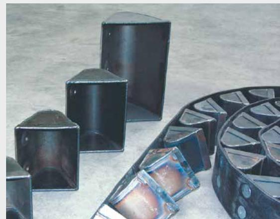
*Bucket elevator belts, buckets and screws for all brands of shot blast machines*
