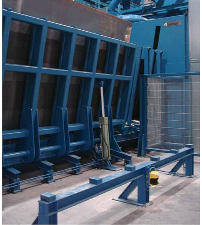
*Vertical roller conveyor shot blast machine*
