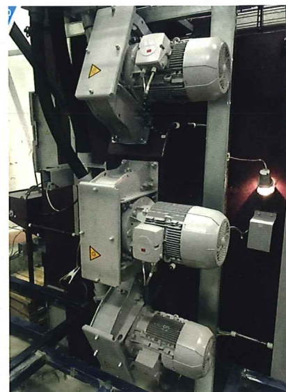
AGTOS turbines with wear parts made of highly wear-resistant hard metal
