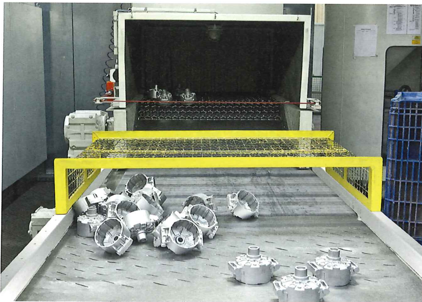
Die-cast aluminium parts leaving a wire mesh conveyor blast machine.
