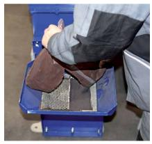
Convenient refilling hopper for the abrasive
