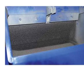
The wind sifter eliminates dust and undersized shot from the abrasive.
