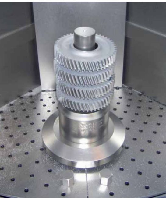
Satellite turntable blast machine for strain hardening of transmission parts
