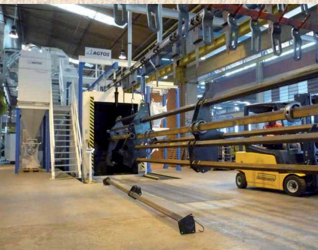
Continuous overhead rail shot blast plant for cleaning welded designs
