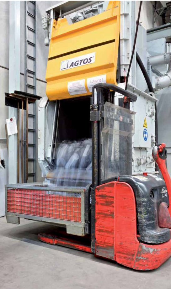
Rubber belt tumble blast machines for shot blasting small parts
