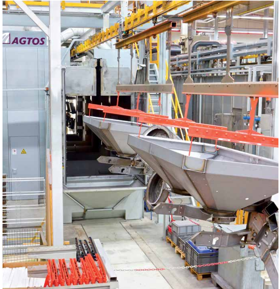
Continuous overhead rail shot blast plant for descaling and cleaning of fertiliser and seed spreaders
