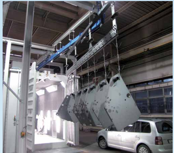
Continuous overhead rail shot blast plant for structural elements
