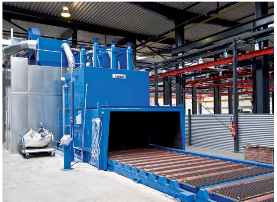
Roller conveyor blast machine for cleaning welded designs
