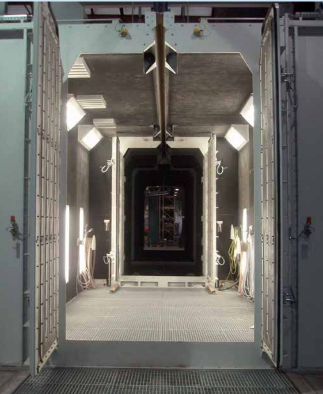
Continuous overhead rail shot blast plant for welded structures with a manual after blast and blow-off room
