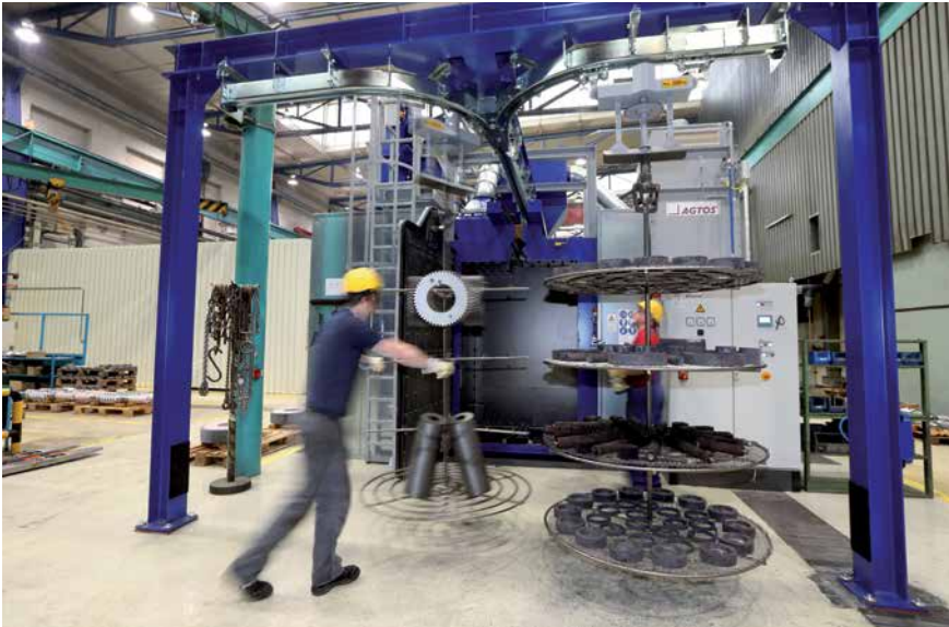
Overhead rail shot blast machine for gear parts as an isolated application
