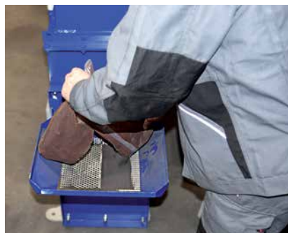
Abrasive refill hopper on the bucket elevator (optional)
