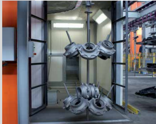
Cast parts exiting the manual blowing chamber of a dual-chamber overhead rail shot blast machine
