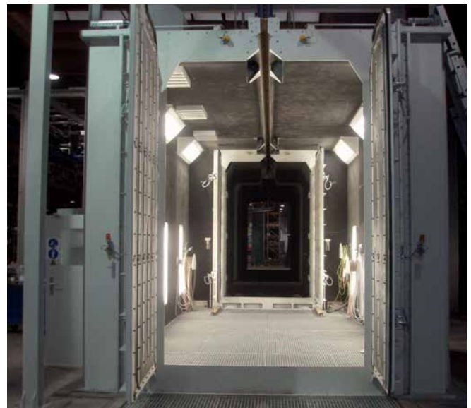
Continuous overhead rail shot blast machine for welded components with manual re-blasting and blowing chamber
