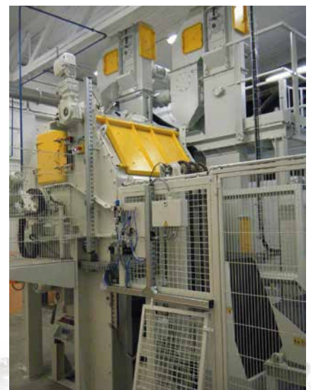
AGTOS drum shot blast machine with a loading device and safety fence
