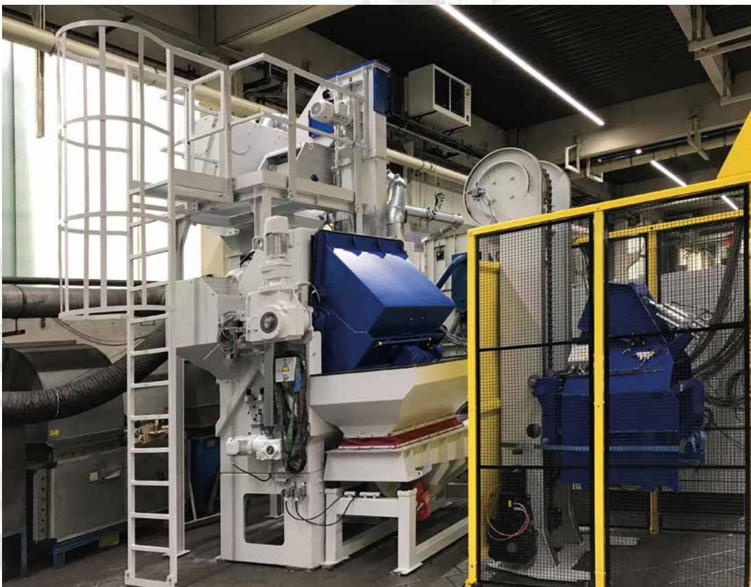
AGTOS drum shot blast machine type TS 150 for cleaning and solidifying small disc springs.
