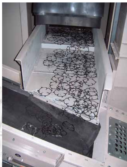
Springs leaving the subsequently installed vibro-chute
