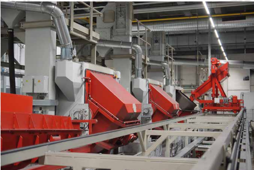
Interlinking the drum shot blast machines enables the continuous production process.
