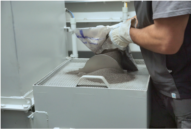
Simple abrasive filling with the refill hopper mounted directly on the bucket elevator
