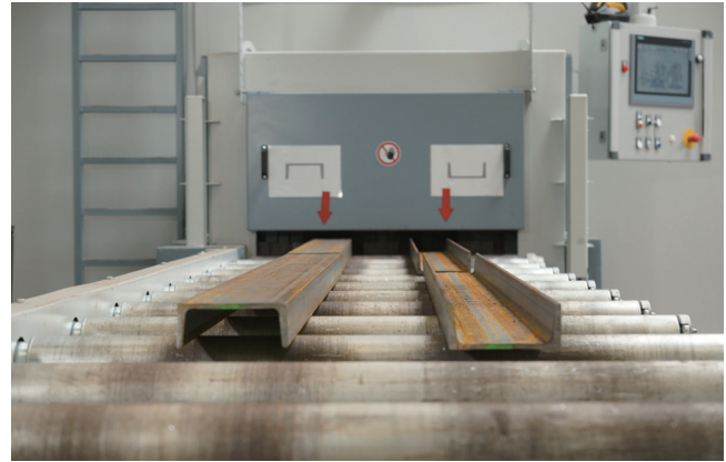
AGTOS roller conveyor blast machine intake for profiles
