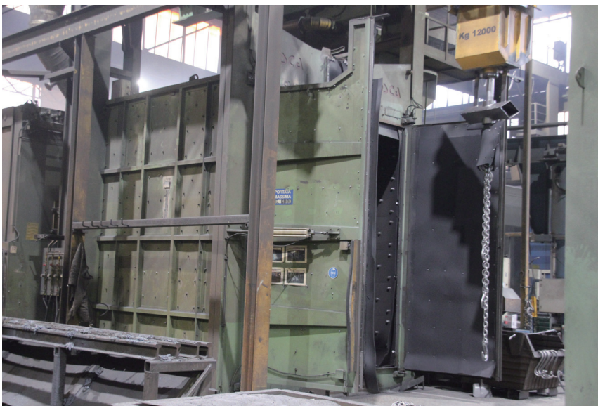
View of the overhead conveyor blasting machine modernized by AGTOS
