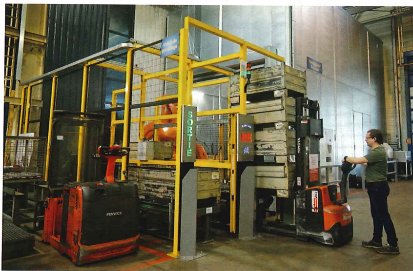
Delivery of new workpiece boxes to the blasting cell
