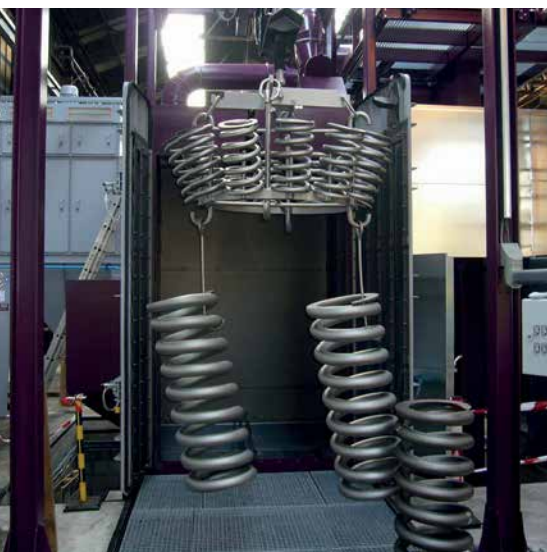
Hanger-type shot blast machine for processing coil springs. The blast chamber measures 1,700 x 1,700 mm.
