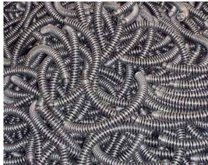
Bow springs after blasting in a rubber belt tumble shot blast machine
