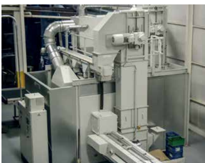
Walking beam shot blast machine for the hardening of long spiral springs
