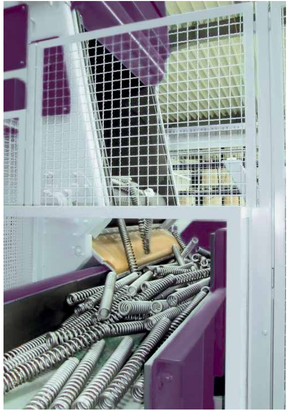
Steel mill tumble shot blast machine for the hardening of coil springs
