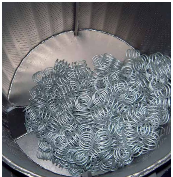
Drum shot blast machine for the hardening of coil springs
