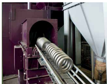
Inlet and outlet of a walking beam shot blast machine for the cleaning of coil springs
