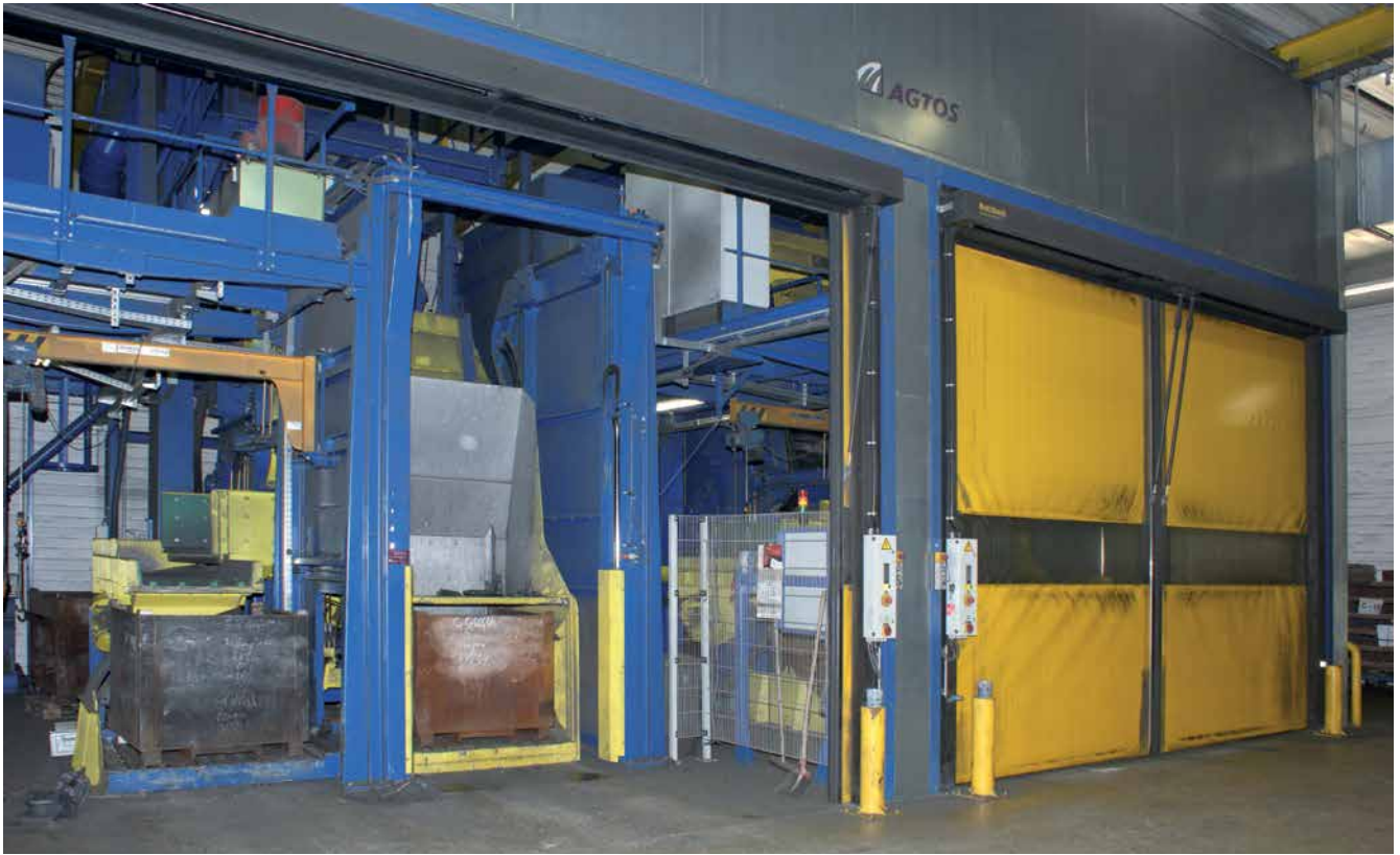
Steel mill tumble belt shot blast machines type MR 850 in twin-operation in a foundry. Quick rolling gates for work safety and noise protection.
