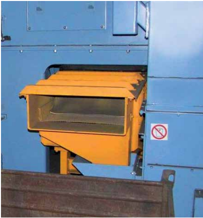
Fig. 1: Vibro chute for discharging coarse particles from the abrasive
