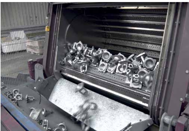
Steel mill tumble blast machine of type MR 0270 for cast workpieces
