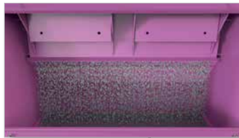
Magnetic/wind sifter for abrasive reclamation
