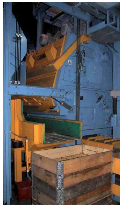
Steel mill tumble belt shot blast machine type MR 850 with loader and vibro chute for processing of castings
