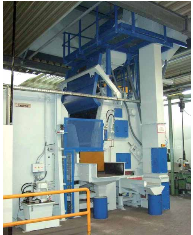
Steel mill tumble belt shot blast machine type MR 750 for shot-peening of springs
