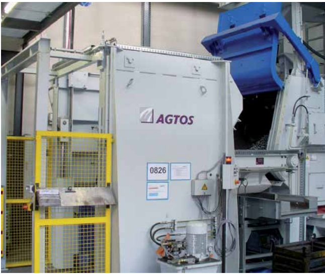
Steel mill tumble belt shot blast machine type MR 550 with loader and vibro chute for processing of engine components
