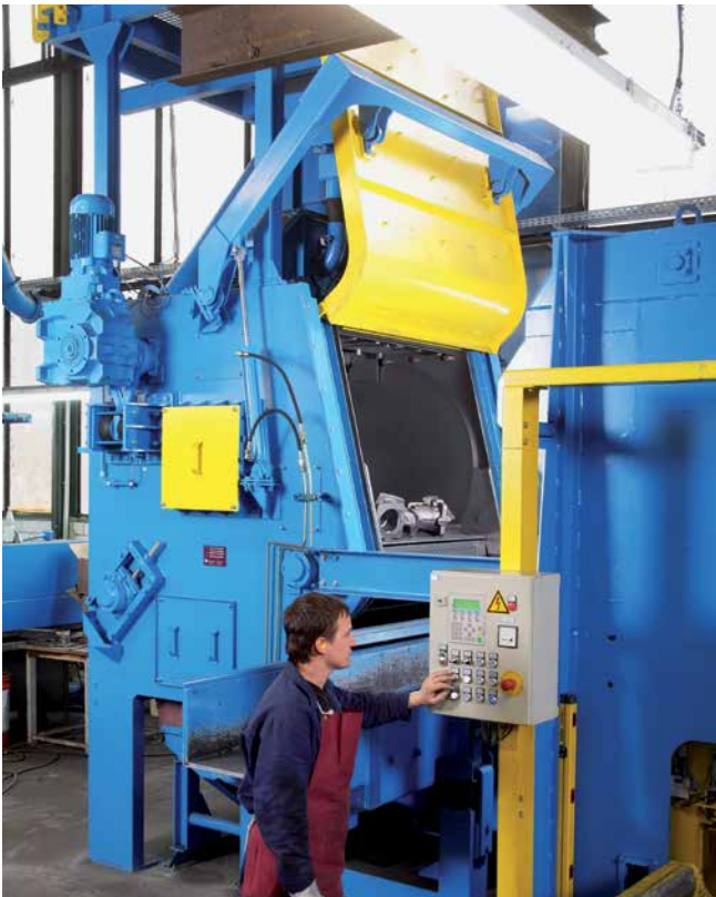
Steel mill tumble belt shot blast machine type MR 550 as a stand-alone solution in a forge
