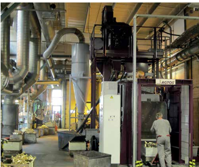
Steel mill tumble belt shot blast machine type MR 270 for blasting armatures
