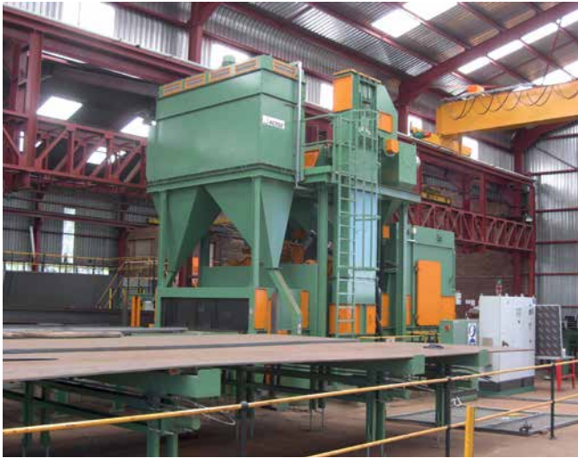
AGTOS RT 26 roller conveyor blast machine for cleaning and descaling plates and sections.
