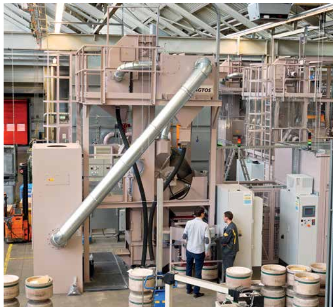
AGTOS drum blast machine in operation
