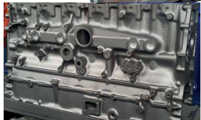
Engine block before and after the blasting process with the AGTOS OCEAN BLASTER
