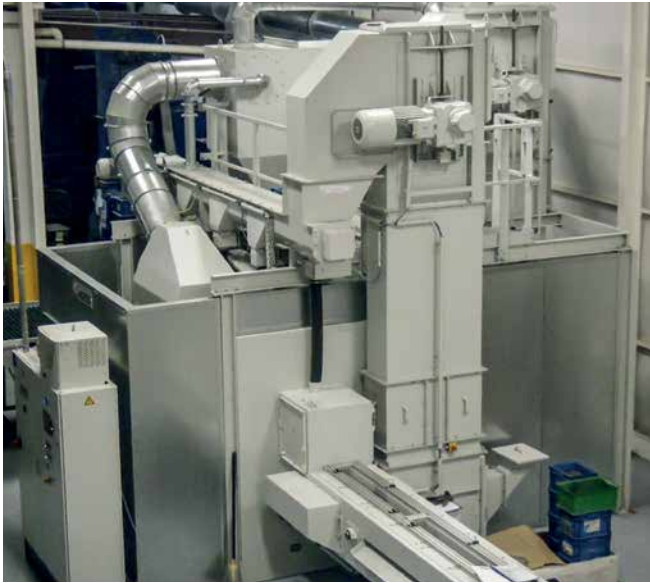
Walking beam conveyor shot blast machine for consolidation of long and stable spiral springs.
