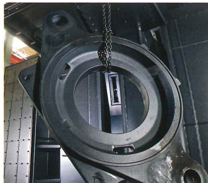
Hanger type shot blast machine for cleaning of big and heavy-weight casted parts.
