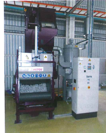
AGTOS rubber belt tumble blast machine for the treatment of mass production parts.
