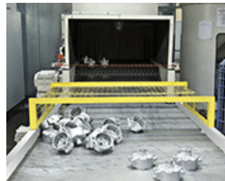
Outlet of an AGTOS-Wire mesh conveyor shot blast machine for aluminum work pieces, Type BS
