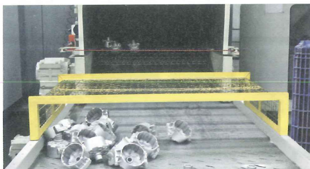
Outlet of an AGTOS-Wire mesh conveyor shot blast machine for aluminum work pieces, Type BS.
