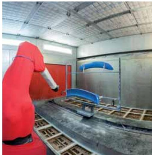
The edrizzi® cubes in this coating booth of the automotive ancillary industry are installed horizontally. The paint mist separators can be used horizontally or vertically, depending on the application.
