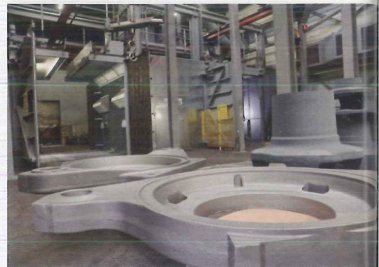
AGTOS shotblast machine for parts with a diameter and height of up to 3.5 metres and a work piece weight of up to 20 tonnes
