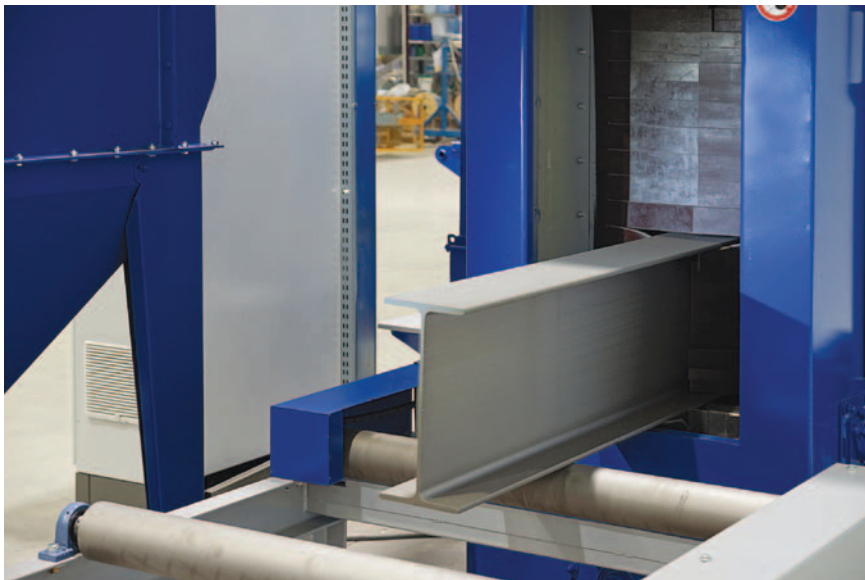
AGTOS Ocean Blaster: Cleaned workpiece is leaving the Ocean Blaster by AGTOS.
