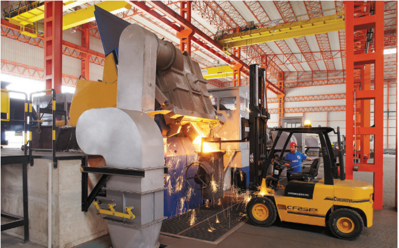
In total the melting shop of Atik Metal consists of three furnaces, each one with two crucibles. Particular capacity: 10 t/h
