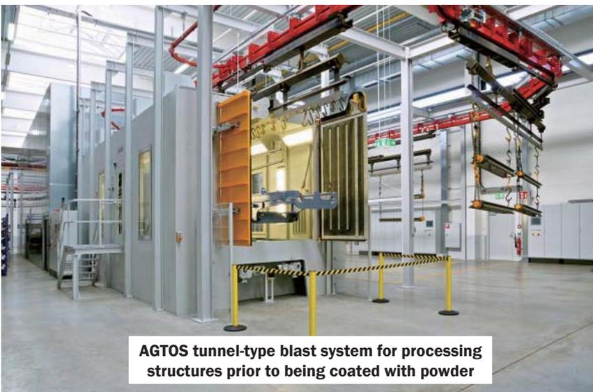
AGTOS tunnel-type blast system for processing structures prior to being coated with powder
