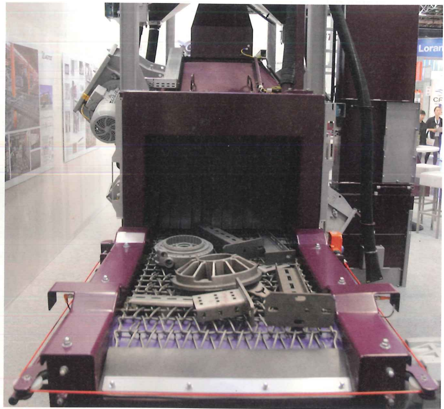
Cast parts in front of an AGTOS wire mesh belt shot blasting machine (Photo: AGTOS)
