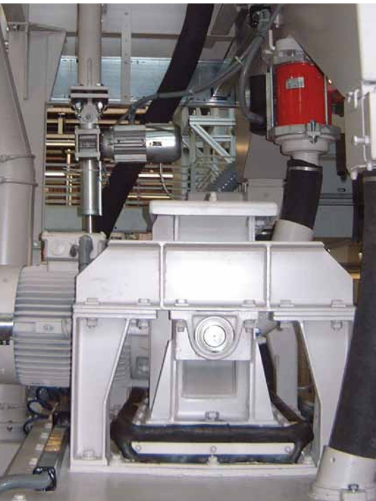
Rotatable AGOS high performance turbine in a satellite turntable shot blasting machine.
