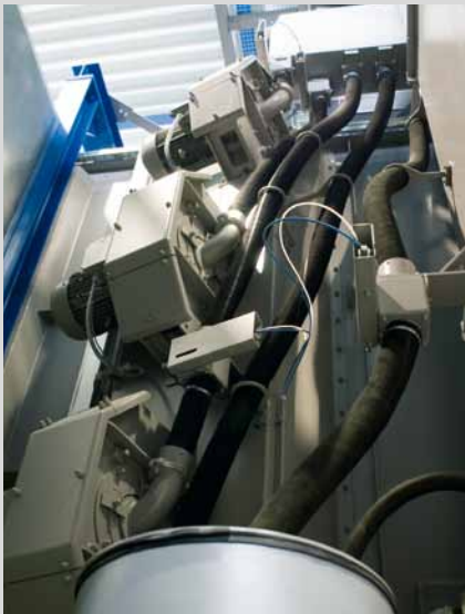
AGTOS high performance turbines installed in a continuous monorail shot blasting machine.
