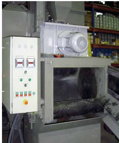
AGTOS high performance turbine in a roller conveyor shot blasting machine (top) and tumble shot blasting machine (bottom).
