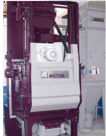
AGTOS high performance turbine installed in a tumble shot blasting machine.
