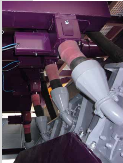
AGTOS high performance turbines installed in a roller conveyor shot blasting machine.
