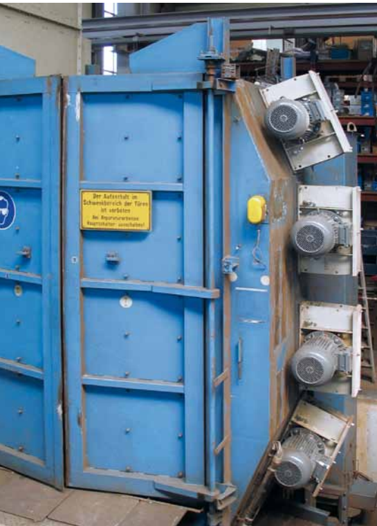
AGTOS high performance turbines are often used to improve the performance of older blasting machines; here: a monorail shot blasting machine.
