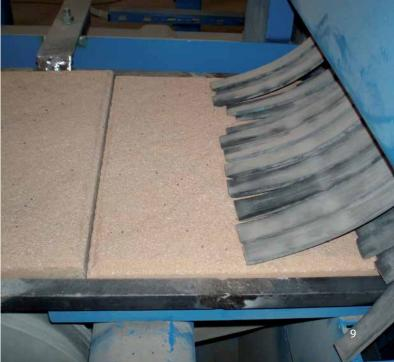
Wire mesh conveyor shot blast machines are used for the treatment of a wide range of work pieces. The advantage is that the parts are blasted from both sides at the same time.
