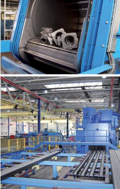
Roller conveyor shot blast machines are used to descale and derust profiles, sheets and fabrications. Using cross conveyors, a roller conveyor system can be linked with individual process steps, such as blasting, preservation, sawing and drilling.
