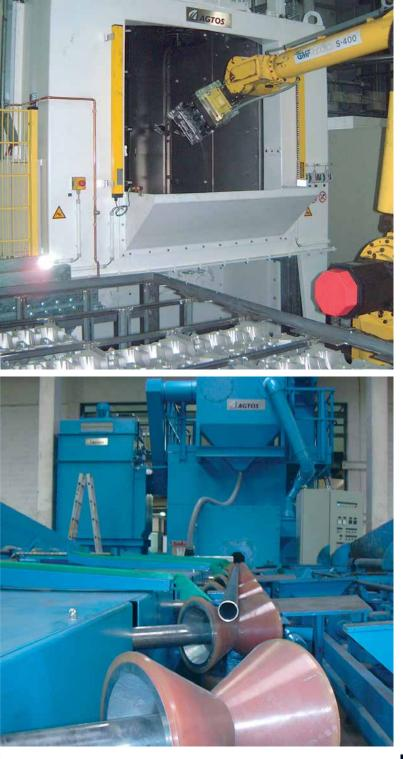
Rotary table shot blasting machines are built in different sizes and designs. For shot-peening the automotive industry prefers to use satellite rotary table shot blast machines. Reduced cycle times and reliable blasting results are the result. In addition, they enable automation of the process.
