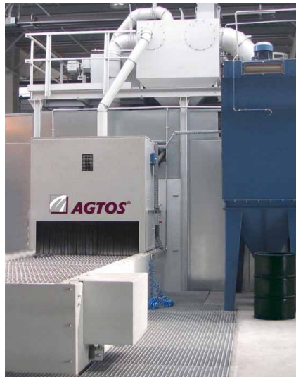
Quick, clean and reliable: AGTOS wire mesh conveyor blast machine with blow-down station and soundproofing
