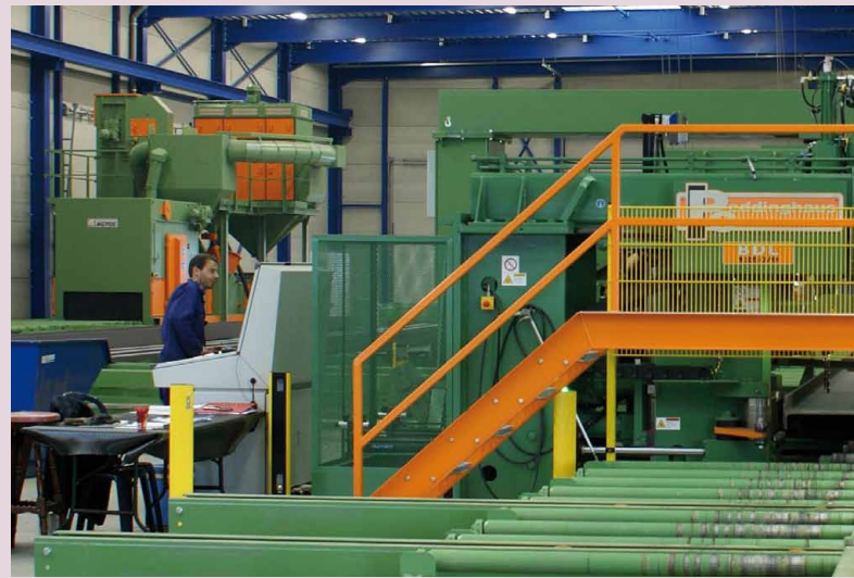
Foreground: the Peddinghaus line of cutting/drilling machines; background: AGTOS roller conveyor blast machine for the treatment of profiles
