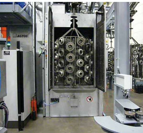
Work pieces on the special device in the blasting machine
