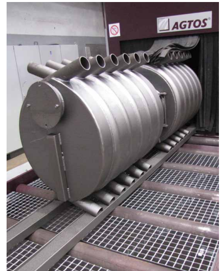
AGTOS construction blast machine for work pieces with complex geometries
