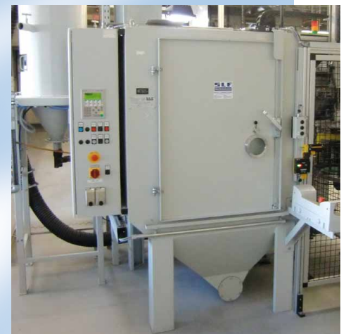
Automatic indexing table unit with direct suction system
