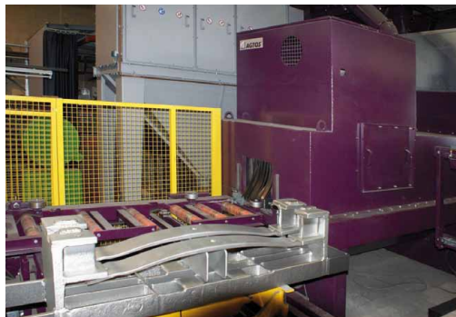
Pretensioned parabolic springs inside the AGTOS blasting machine.
