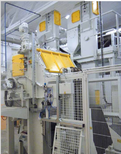
AGTOS drum blast machine with feeder
