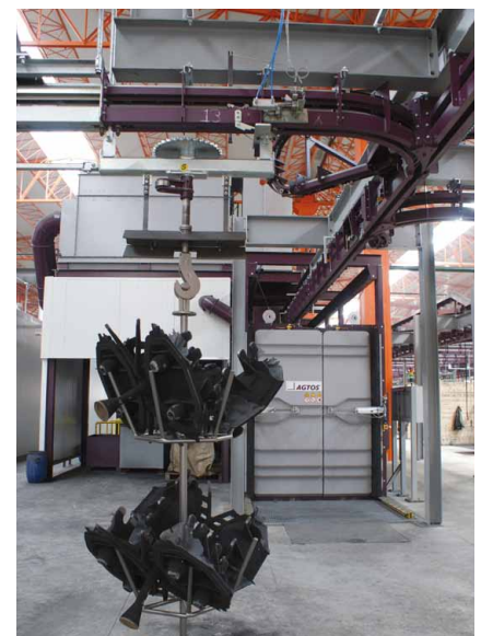
Castings with sand adhesions before the blasting process
