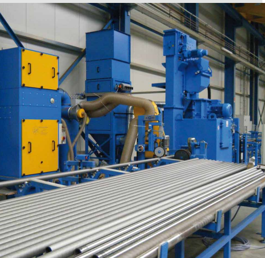
AGTOS Diabolo Pipe Blast Machine for cleaning pipes with a diameter of 60 to 160 mm.
