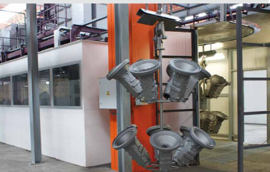
Exit ramp of the blasting machine with jet-cleaned castings
